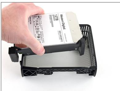
Remove the hard drive from the frame.
