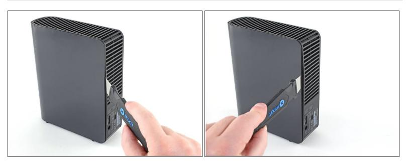
Slide the Jimmy up along the seam and pry the frame outward to release the top plastic clip.
