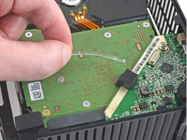
Slide the LED light guide out of the LED slot on the drive's controller board.
