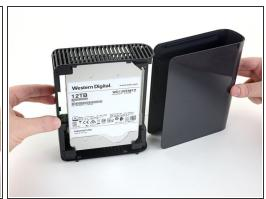
Slide the cover straight off the frame to remove it.
