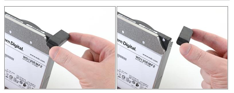
Remove the rubber blocks from the hard drive if they're still attached—some of them may have already fallen off when you removed the hard drive.
