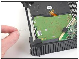
• Grab the end of the LED light guide and slide it completely out of the frame to remove it.
