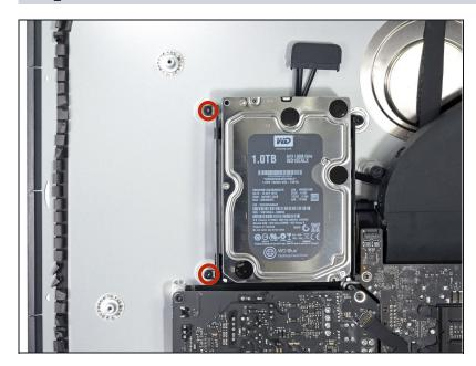
Remove two 7.3 mm T8 screws securing the left hard drive bracket to the rear case.
