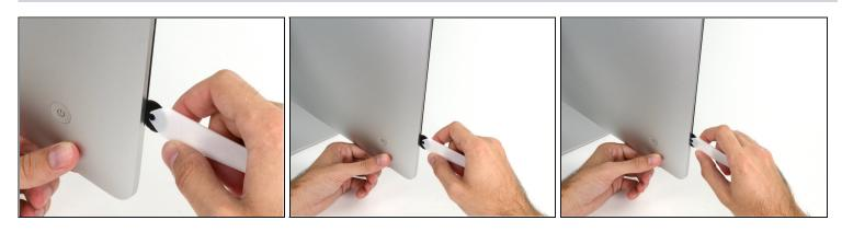
Starting on the left of the display, near the power button, insert the iMac Opening Tool
