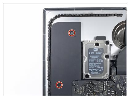
Remove two 10 mm T10 screws.
