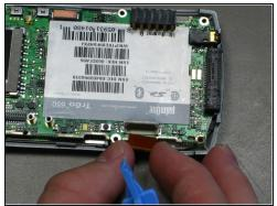
⚠ Disconnect the ribbon cable before removing the motherboard.
