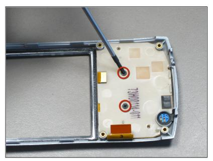
Unscrew the two 3.2 mm screws with a Phillips #00 screwdriver.
