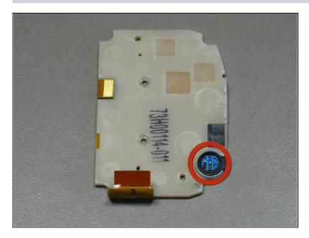
Place the circuit board with the microphone facing up.
