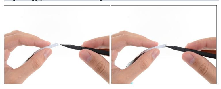
• Insert the tip of a spudger into the hole at the end of the strip where you just removed one layer of backing. Insert the spudger from the side that still has a layer of white backing on it.
