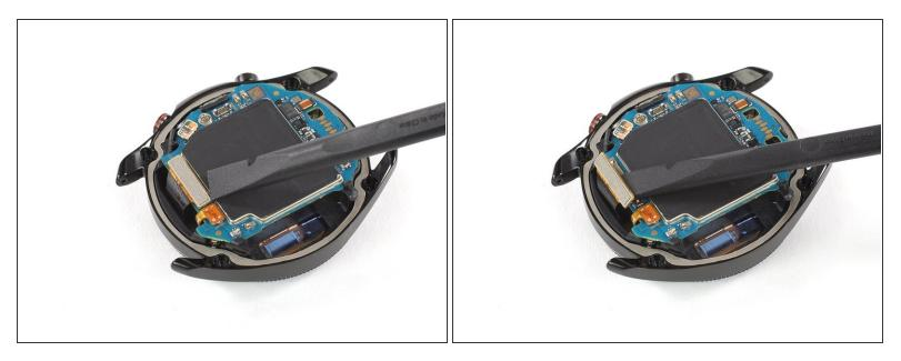
• Use the flat end of a spudger to pry up and disconnect the display flex cable from the motherboard.
