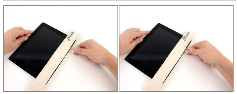
• Remove the plastic opening tool from the iPad, and push the opening pick further underneath the front glass to a depth of ~0.5 inches.
