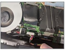
• Gently pull the white battery connector out towards the battery.
