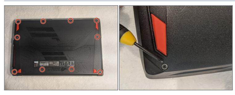
Use a JIS screwdriver to remove the ten 4 mm screws from the bottom cover.
