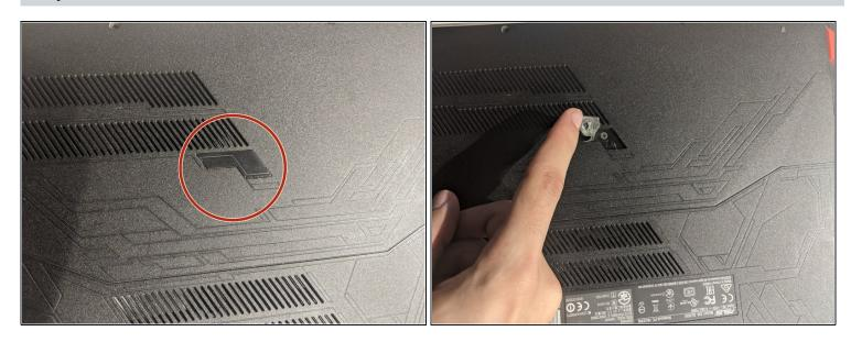
Open the flap in the middle to reveal the 11th screw and remove it using the same JIS screwdriver.
