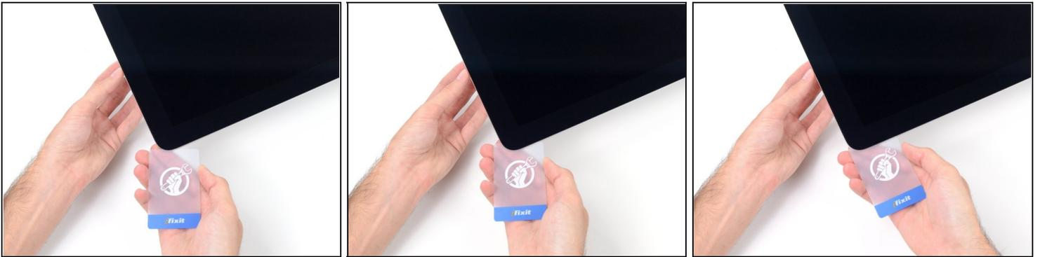
ⓘ While the opening tool did the lion's share of the work, the display will still be slightly adhered to the case. A [plastic card](#) will be necessary to free up the last of this adhesive.
