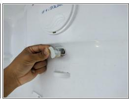
Using a spudger, pry off the cap covering the topmost screw.
