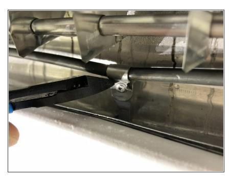
Cut out the old evaporating clip using a pair of cutting pliers.
