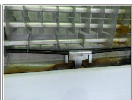
Replace the old clip with a new evaporating clip.
