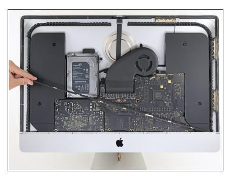
Remove the lower support bracket (a.k.a. "chin strap") from the iMac enclosure. To reassemble your device, follow these instructions in reverse order.
