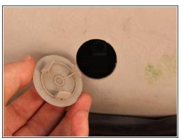
• Use the flat head screwdriver to pry off the small round access panel on the interior of the tailgate.
