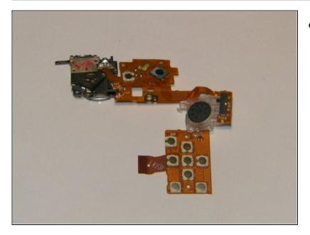
• The rear control board should now be completely separate from the camera.
