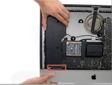
Lift the left speaker straight up, until the power button cable is exposed (about 0.5").
