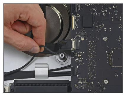
De-route the left speaker cable by pulling it straight up out of the retaining clip in the back of the rear enclosure.
