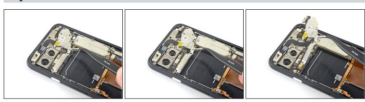
• Using a pair of tweezers, tilt the camera cover up and slide it out of the retaining slot on the upper right corner of the phone to remove.
