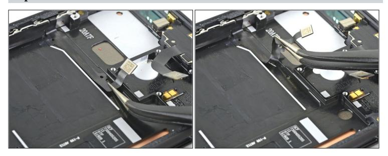
• Use a pair of tweezers to peel the side button flex cable off of the phone's frame. It is secured with some light adhesive.
