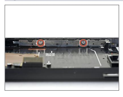
Use a T3 Torx driver to remove the two 2.4 mm screws securing the button bracket to the frame.
