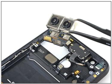
Use a pair of tweezers to remove the rear-facing camera module.
