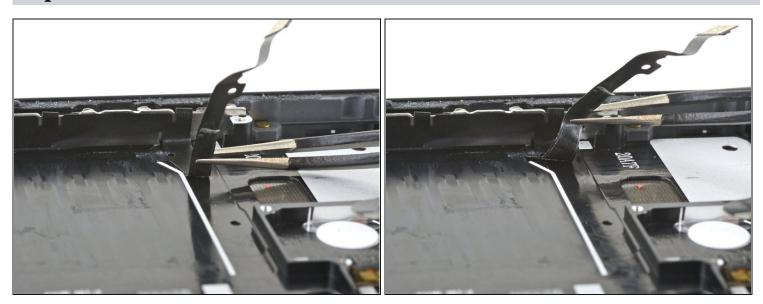
• Continue peeling the flex cable until it is no longer adhered to the back side of the phone.
