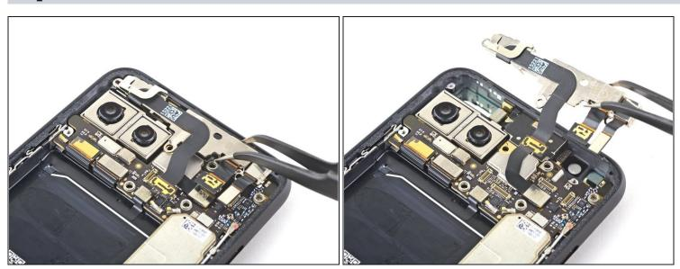
Use a pair of tweezers to remove the front camera and sensor assembly.
