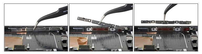
• Use a pair of tweezers to remove the button bracket.
