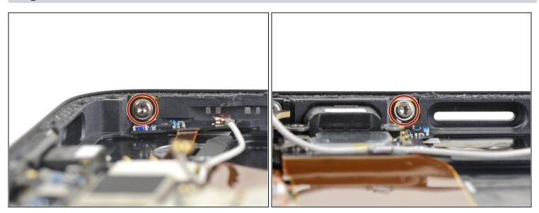
• Use a T3 Torx driver to remove the two 2.1 mm screws securing the charging assembly to the frame, one on the left side and one on the bottom side.
