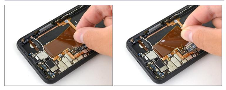
• Peel back the ribbon cable that's adhered to the phone's frame. It's secured with some light adhesive.
