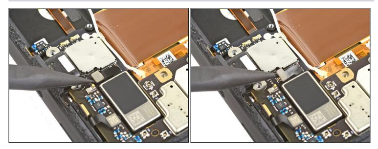
• Disconnect the vibration motor connector from the charging assembly.
