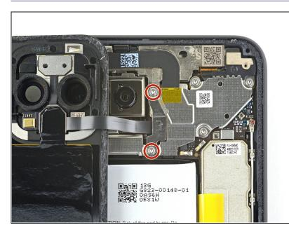
• Use a T3 Torx driver to remove the two 4 mm screws securing the back panel connector cover.
