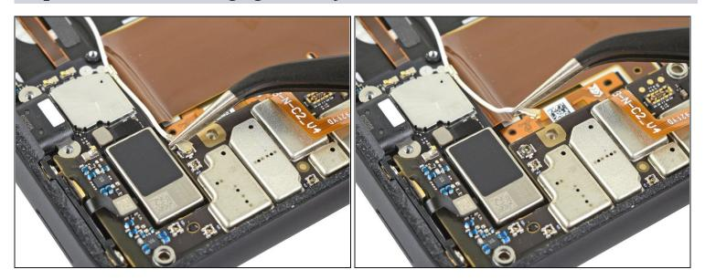
• Use a pair of tweezers to disconnect the <u>antenna press connector</u> from the charging assembly by pulling it straight up from the motherboard.
