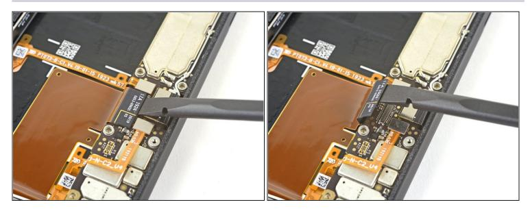
• Use the flat end of a spudger to disconnect the charging cable connector by prying it straight up from the motherboard.
