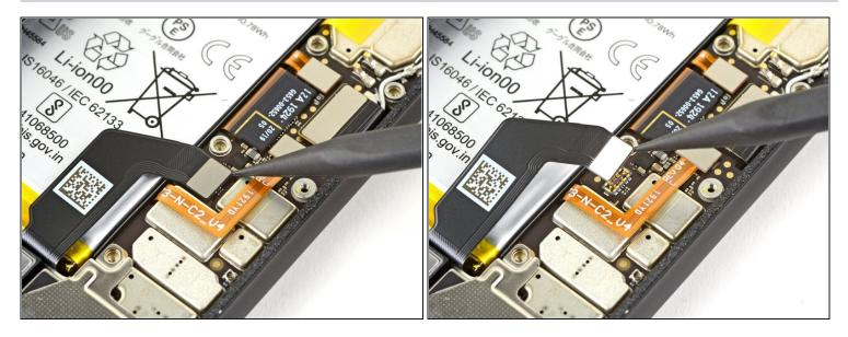
A Whenever you use the spudger near the battery, be very careful not to puncture the battery.
