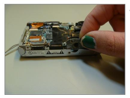
• Remove tripod piece located at the bottom of the camera. This piece should slide out with ease.
