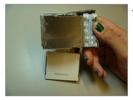
• The LCD is now removed from the camera, although attached by a ribbon at the bottom of the camera.
