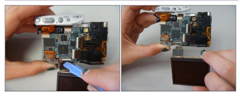
• Use pry stick to pop out LCD connector ribbon, also called the ZIF connector.
