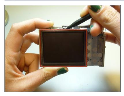
• Use the spudger to pry the LCD from the camera.
