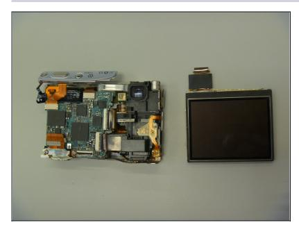
• The LCD is now removed from the camera.
