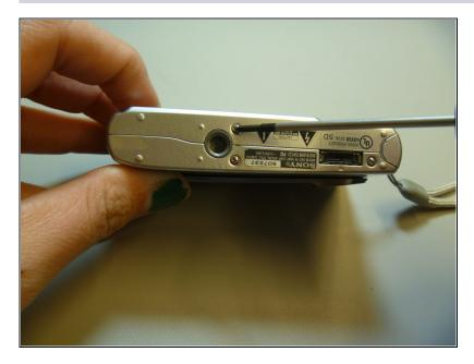
• Use screwdriver to remove screws.
