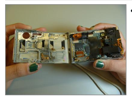
• The front cover is now removed from the camera and the internal hardware is now exposed.
