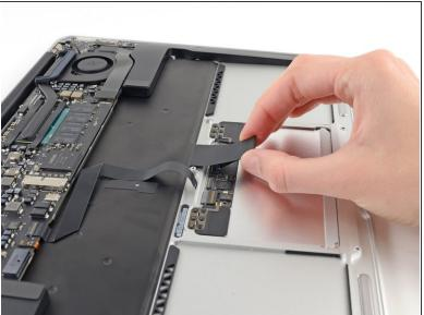
While carefully lifting the keyboard ribbon cable with one hand, use the tip of a spudger or your fingernail to flip up the retaining flap on the keyboard ribbon cable ZIF socket.
