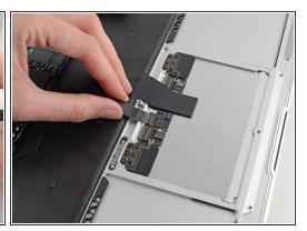
• Use the tip of a spudger or your fingernail to flip up the retaining flap on the trackpad ribbon cable ZIF socket.
