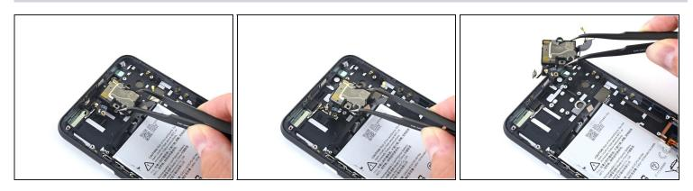
Use a pair of tweezers to remove the earpiece speaker and Soli motion sensor assembly.
