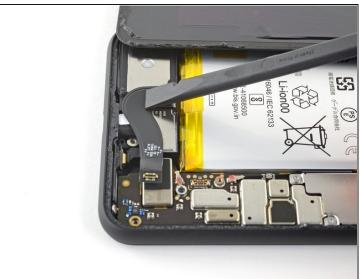
Using the flat end of a spudger, gently fold the battery cable over so it doesn't accidentally
