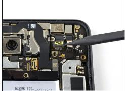
Using the pointed end of a spudger, pry the camera and sensor connectors straight up from the motherboard.
