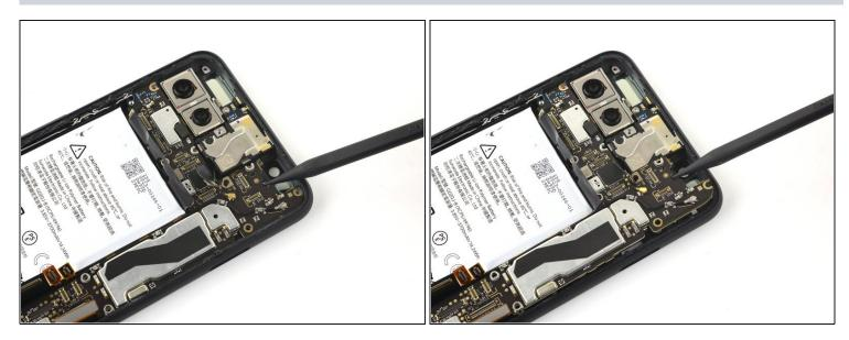
Using a spudger, pivot the top end of the motherboard up and out of the phone's frame.
