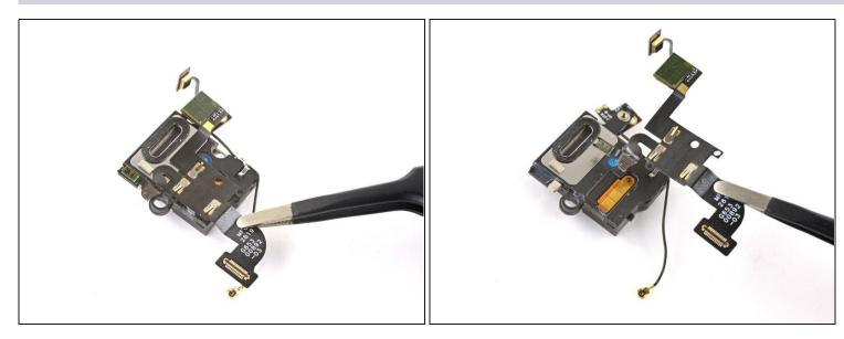
Use a pair of tweezers to peel away and remove the Soli motion sensor cable, which is held in place with some light adhesive. Compare your new replacement part to the original part—you may need to transfer remaining components or remove adhesive backings from the new part before installing.
