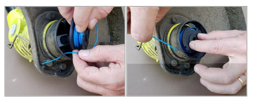
Thread the replacement reel line into the hole and push the replacement reel in.
