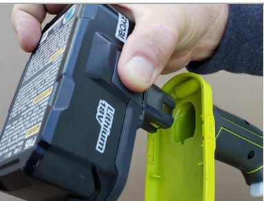
Press the button and pull to remove the battery.
