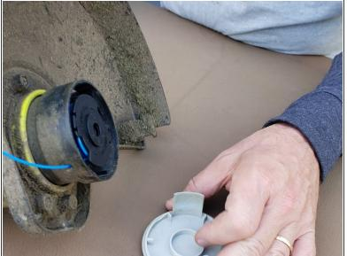
Press the button and pull to remove the line cover.
