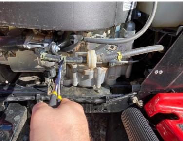
Using your pliers, slide the metal clip located on the left side closest to the filter down the fuel line.
