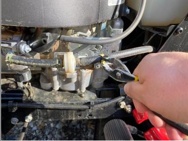
Slide the metal clip located on the right side closest to the filter, using your pliers, and slide the clip down the fuel line.
