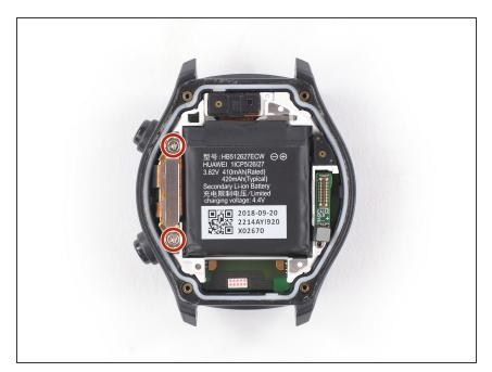
Remove the two Phillips #00 screws (1.8 mm length).
