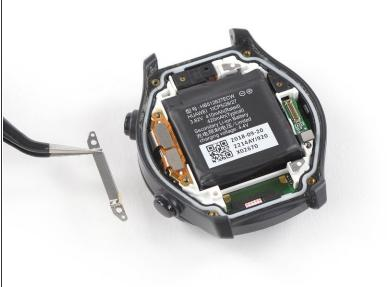
• Use a pair of tweezers to remove the metal shield covering the display and the digitizer flex cables.
