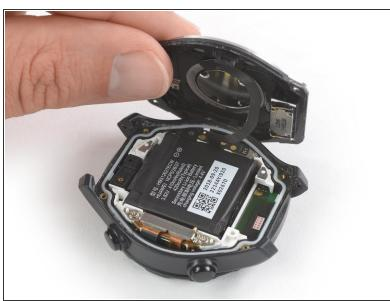
Carefully fold the back cover assembly to the opposite side of the two watch crowns.
