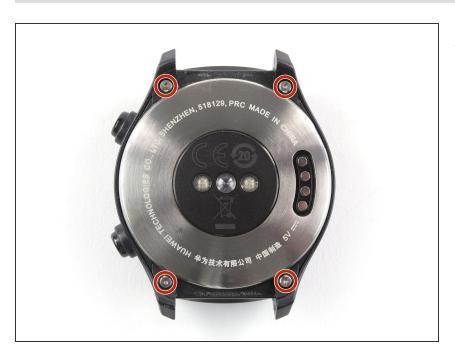
Remove the four Torx T2 screws (4.5 mm length).
