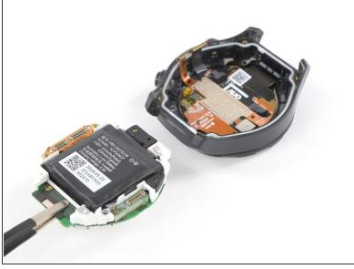
Use a pair of tweezers to remove the battery and motherboard assembly.
