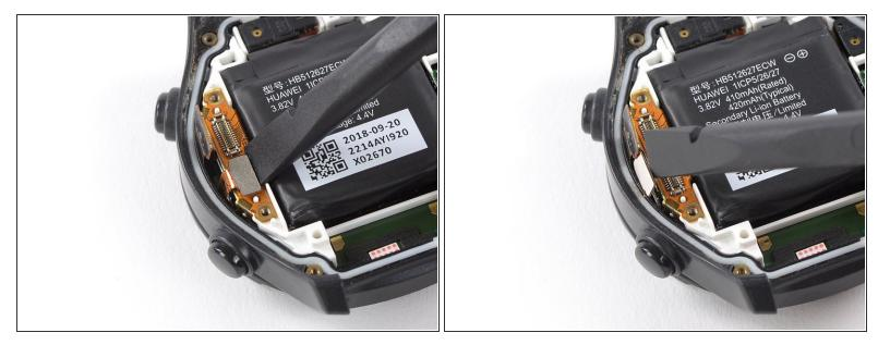
• Use the flat end of a spudger to pry up and disconnect the display flex cable.
