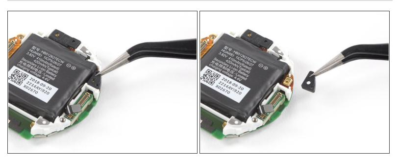
Use a pair of tweezers to remove the black rubber gasket from the microphone next to the top right corner of the battery.
