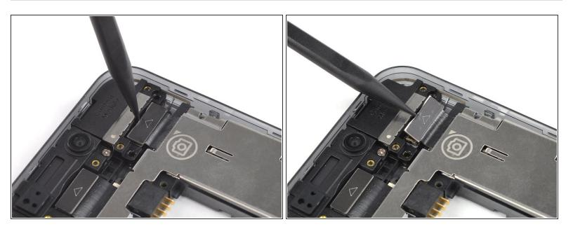
• Use a spudger to pry up and disconnect the camera connecting cable.
