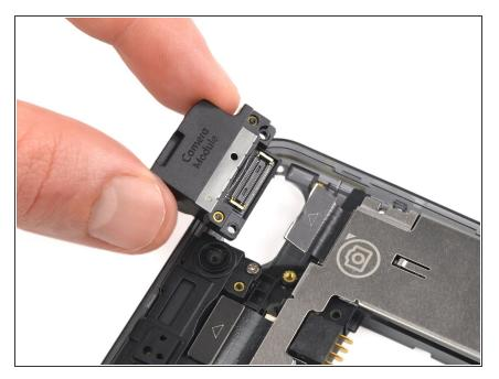
Remove the rear camera module.
