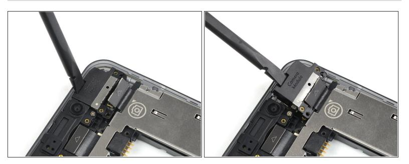
Use a spudger to pry up the rear camera module.
