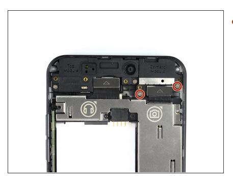
Remove the two 4.1mm-long Phillips #00 screws.
