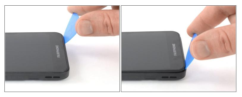
Slide the opening pick around the bottom right corner and use it to disengage the plastic clamps at the bottom of the display module.
