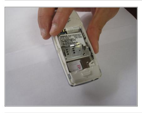
Once the SIM card compartment has been opened, insert the SIM card into the slot provided on the left side.
