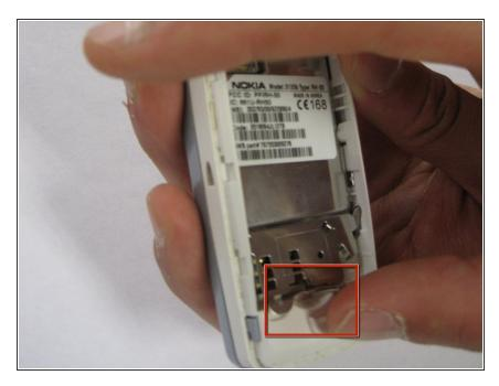
Once the battery is removed, the SIM card compartment will be exposed. Pry the compartment open as seen in the figure. This can be done using your fingernail or a prying mechanism.
