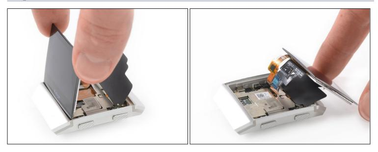
Carefully fold the display assembly onto the upper side of the watch.
