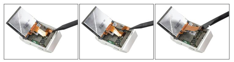
• Use a spudger to pry up and disconnect the two display cables from the motherboard.
