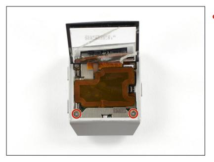
• Remove the two Torx T2 screws (3.65 mm length) from the top edge of the watch.
