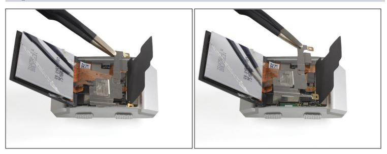
• Use a pair of tweezers to remove the metal cover.
