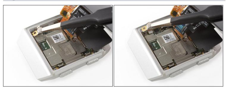
• Use a pair of <u>tweezers</u> to remove the metal shield covering the battery flex cable.
