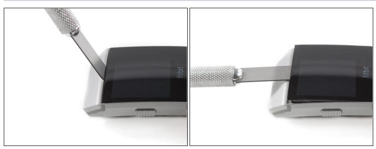
• Use a technician's razor with a flat blade to pry up the top edge of the display and create a small gap.
