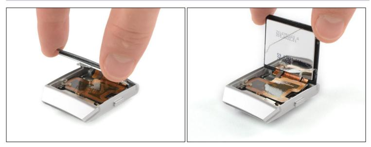
• Carefully fold the display assembly in the direction of the bottom edge.
