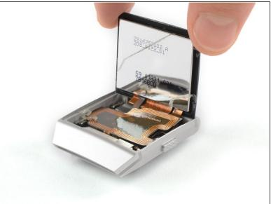
Carefully fold the display assembly in the direction of the bottom edge.
