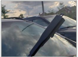
Look for a clip/tab on the top of the wiper blade. Push the tab until it slides out of the metal arm and then the wiper blade should come right out of the metal arm.
