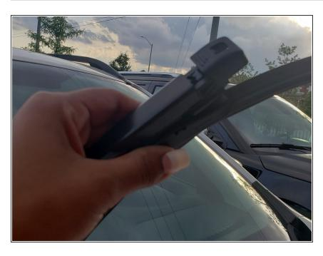
The top of the adapter has a tiny black housing. Fit the top of the wiper arm into the housing and align the bottom of the adapter with the tabs on the arm. Press firmly until you hear a click. Finally the wiper blade is installed.
