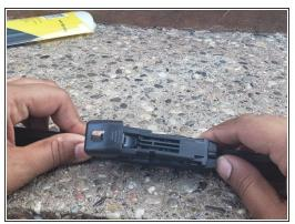
• Install the new adapter ensuring the connector aligns with the blade assembly. The adapter must click for a secure fit.
