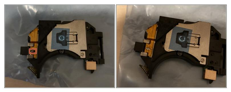
Most of the lasers have some solder on it for the anti-static security. You NEED to remove the solder, otherwise it won't work. Remove the solder with desolder wick.
