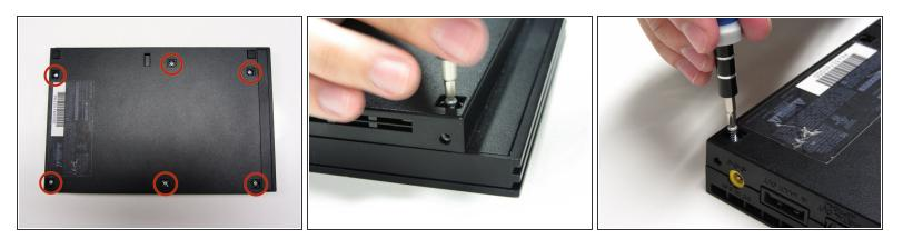
• Remove all six 4.0 mm screws from the base of the unit using a #1 Phillips screwdriver.
