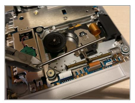
Remove the slider as shown in the picture. You could do this with your fingers, otherwise take tweezers to remove it.
