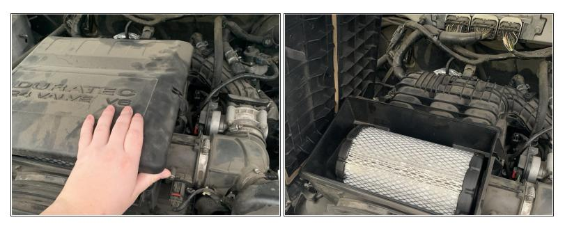
Remove the cover of the air filter compartment, exposing the air filter.
