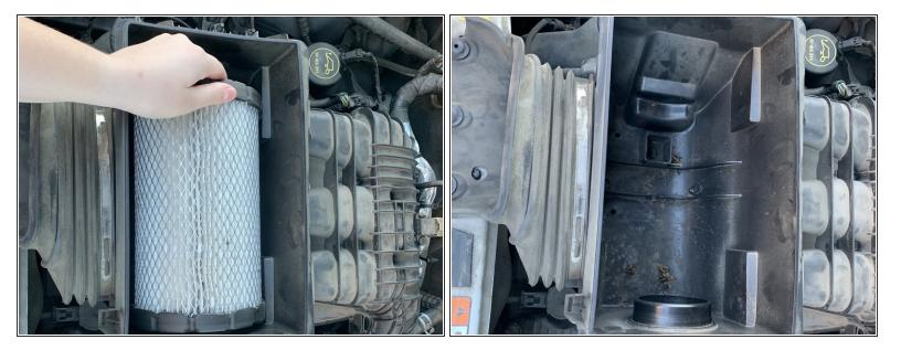
Take out the air filter, by lifting up and to the left.
