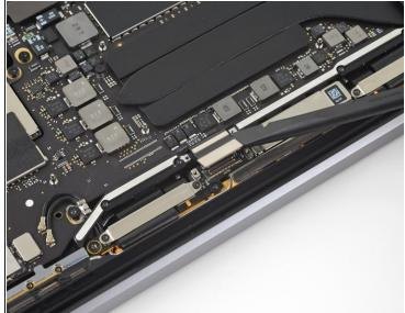
• Pry the display board flex cable straight up from its socket to disconnect it from the display board.
