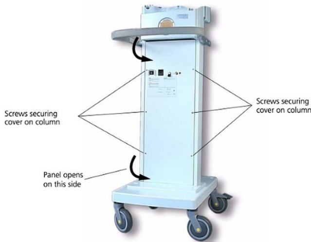
Figure 11-3. Positions of the screws securing the rear panel on the column
