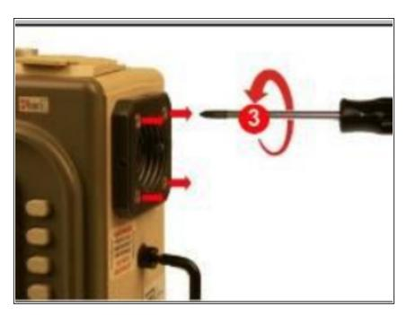
Loosen but do not remove the(4) 8-32 X 3 screws on the outer air intake.
