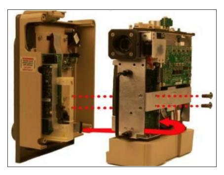
Place the front case assembly over the vent module and tighten the (2) 4-40 X 1/4 screws unto the dovetail mounting bracket. Reconnect the ribbon cable unto the PIM PCB. Make sure the two locking "ears" lock into position.
