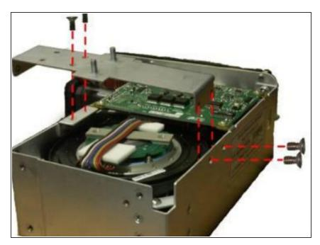
Install the dovetail stabilizer bracket ontothe new SPM assembly by tightening the (2) 6-32 X <sup>1</sup>/<sub>4</sub> and (2) 4-40 X <sup>1</sup>/<sub>4</sub> screws.
