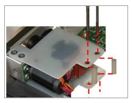
Secure the Power Input assembly to the Chassis using the (2) spacers and (2) 4-40 X 1 ¼ screws. Do not over-tighten the screws.
