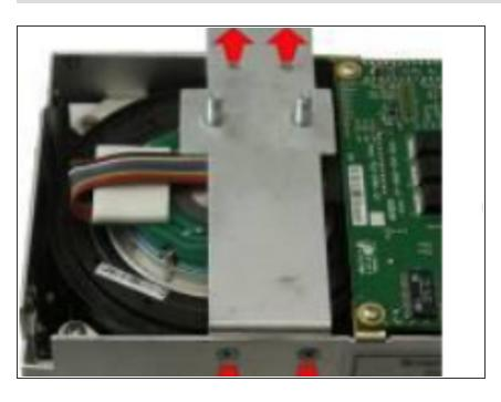
Remove the Dovetail stabilizer bracket by loosening and removing the (2) 6-32 x ¼ and the (2) 4-40 X
