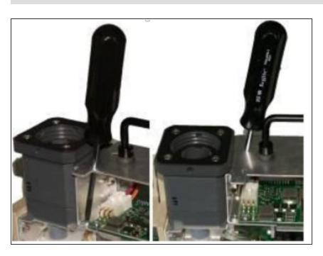
Insert screwdriver through the holes on the chassis to loosen and remove the (2) 6-32 x 5/16 screws holding the chassis to the vent module.
