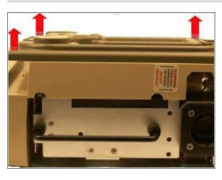
Flip the ventilator over and remove the front case assembly by lifting it straight up away from the ventilator module.
