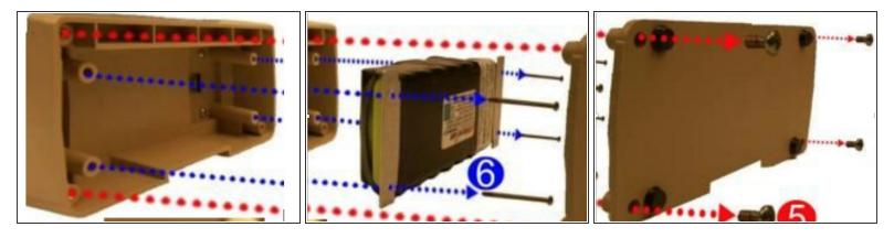
Remove the battery compartment cover by unscrewing the (4) 6-32 X 5/16 screws.
