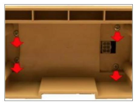
Unscrew the (4) 6-32 X 5/16 Phillips screws to remove the damaged battery compartment case.
