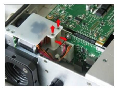
Loosen and remove the (2) 4-40 X 1
