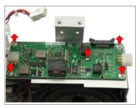
Remove the PIM PCB by loosening the (5) 4-40 X 5/16 screws.
