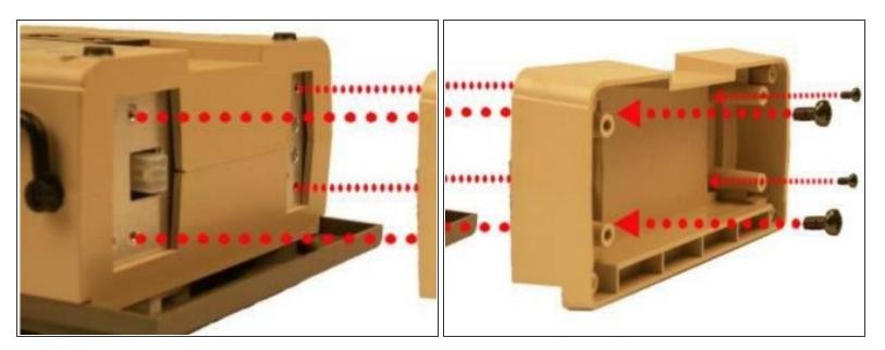
Rotate battery compartment to mate with upper and lower case cutouts and press firmly into place.
