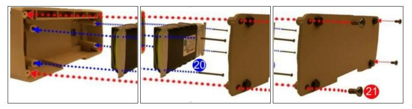
Re-assemble the battery compartment cover by tightening the (4) 6-32 X 5/16 screws.
