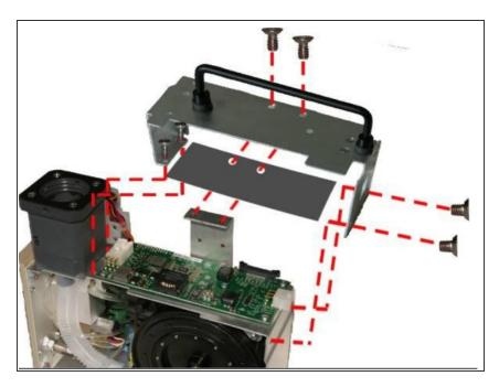
Secure the chassis to the vent module using the (2) 6-32 X <sup>1</sup>/<sub>4</sub> screws with SPO2 insulator, the (2) 8-32 X <sup>1</sup>/<sub>4</sub> and the (2) 6-32 x 5/16 screws.
