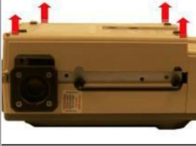
Loosen and remove the (2) 10-32 Keps nuts and the (4) 6-32 X 2 screws. Remove the back case by lifting from the ventilator.
