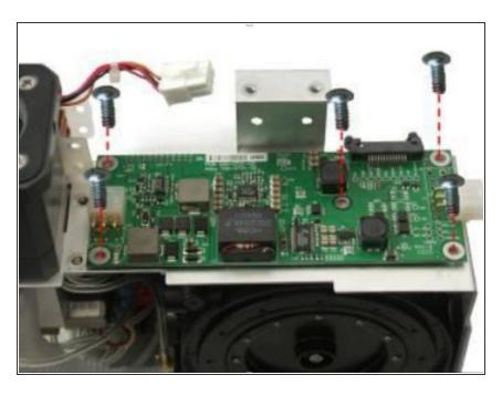
Secure the PIM Board to the new SPM with the (5) 4-40 x 5/16 screws.
