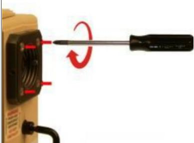
• Tighten the (4) 8-32 X 3 screws on the outer air intake.
