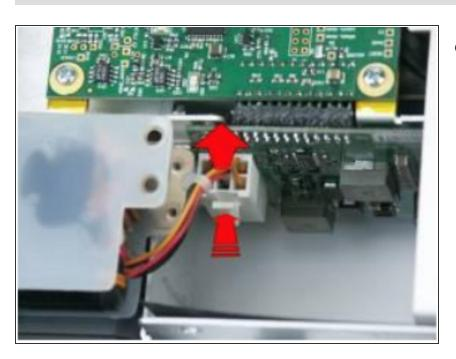
Disconnect the Power Input cable from the PIM PCB by pressing on the locking latch and pulling the cable straight up from the connector.
