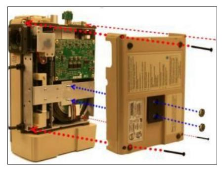
Attach the back case to the vent module and align cover with handle, air intake housing and dovetail mounting studs. Insert and tighten the included (2) 10-32 Keps nuts and the (4) 6-32 X 2" screws.
