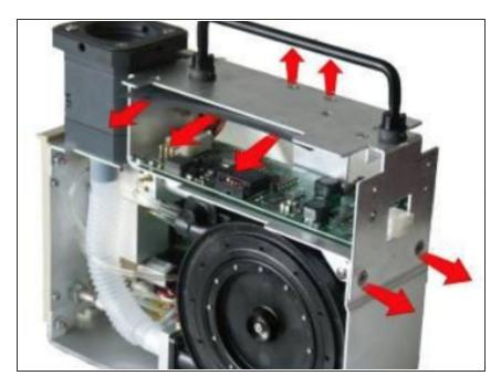
Loosen and remove the (2) 6-32 X ½ screws holding the chassis to the dovetail mounting bracket and remove the SPO2 insulator. Loosen and remove the (2) 8-32 X ½ screws holding the chassis to the vent module
