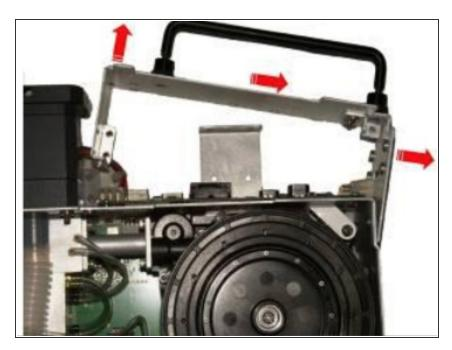
Lift the damaged chassis from the ventilator module.
