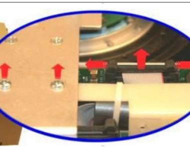
Remove the (2) 4-40 X ¼ screws on the Dovetail Mounting Bracket and disconnect the ribbon cable on the PIM PCB by simultaneously applying pressure on the two locking "ears".
