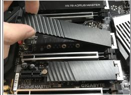
• Unscrew the opposite end of the M.2 cover and gently pull diagonally to reveal the SSD slot.
