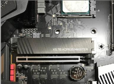
• Use the computer supplied (2.0 x 3.0 mm) Phillips #0 screw to secure the SSD dust cover.
