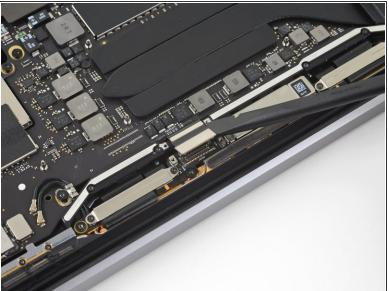
Pry the display board flex cable straight up from its socket to disconnect it from the display board.
