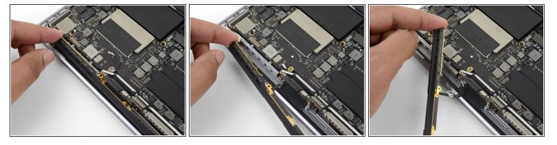
Carefully remove the antenna assembly, while simultaneously feeding the antenna cable bundle through the hole in the chassis.
