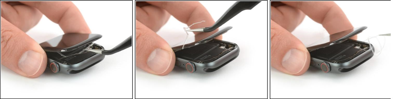
**⚠ To avoid straining the display cables, don't open the display all the way yet.**
