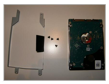
The hard drive is now removed from the caddy and the replacement can be installed.
