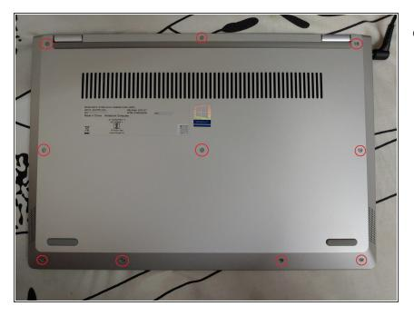
Take out the 10 Torx T6 screws as marked and pry open the back cover. I pried from the top (midpoint of the chassis in between the two hinges) as it felt easier that way. You can use a prying tool for completion of this step.
