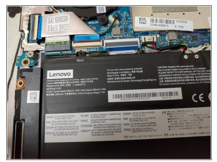
Battery details: 2965 mAh/45Wh, 15.36V - 17.6V
