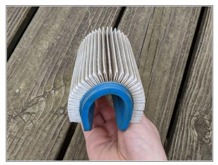
• Lightly bend the filter so that you can see all surfaces of the filter.
