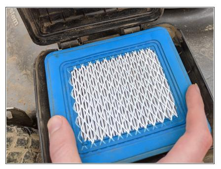
• Make a note of the position of the filter, and remove the cover.
