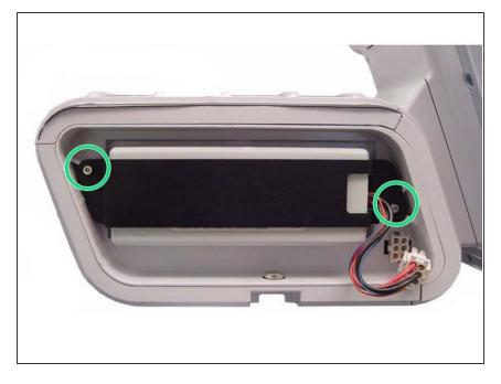
Using a 3-mm hex wrench, remove the battery bracket by removing two screws.
