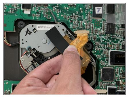
• Disconnect the ribbon cable by pulling it straight out of the connector.
