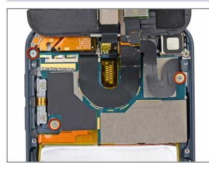
• Remove three 1.6 mm #000 Phillips screws securing the logic board to the rear case.
