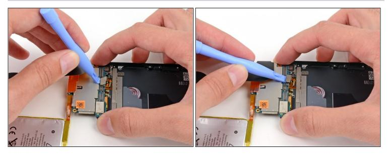
• Use the edge of a plastic opening tool to disconnect the display connector from the back of the logic board.
