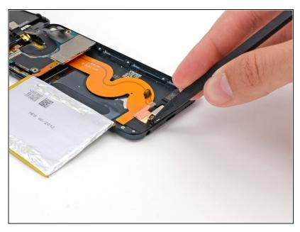
• Use the tip of a spudger to peel back a small piece of tape covering a screw on the left side of the headphone jack.
