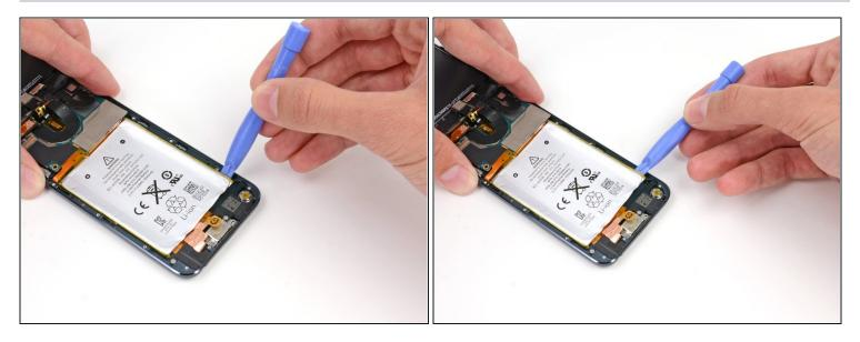
• Continue with the lower right notch. Insert the plastic opening tool into the notch, and gently pry up on the side of the battery.
