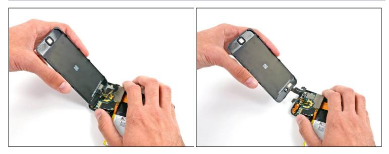
• Remove the display assembly from the iPod.
