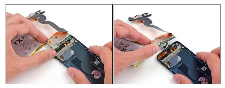
• Remove the logic board assembly from the rear case of the iPod.
