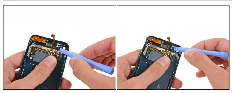
• Use a plastic opening tool to pry the microphone up from the rear case.
