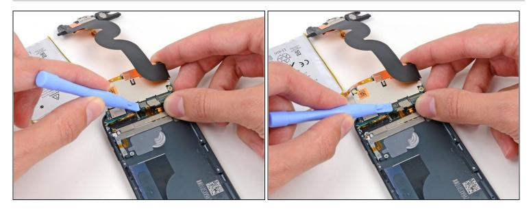
• Disconnect the button ribbon cable connector from the back of the logic board.
