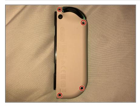
Using the Y00 Tri-Point screwdriver, remove four M1.4 x 5mm screws to loosen the hard plastic back of the Joy-Con.
