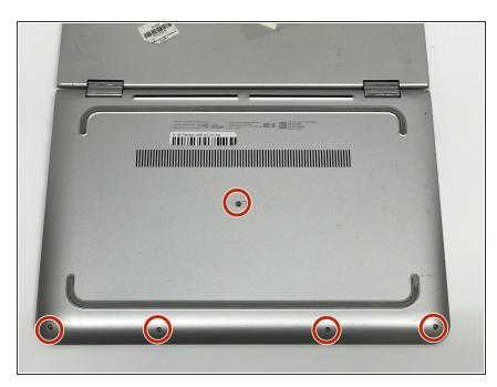
Remove five 1.4mm Phillips #1 screws from the bottom of the laptop.
