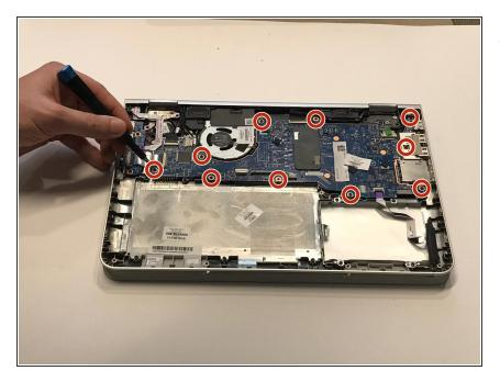
Remove the ten 1.2mm Phillips #1 screws that hold the motherboard into the frame of the laptop.
