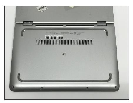
• Flip the laptop over so that the bottom of the laptop is facing up.
