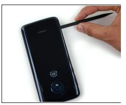
• Insert a spudger into the lower half of the left side of the phone about 2 cm and slide it down the left edge to release the left strip of adhesive.
