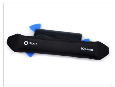
Heat the left edge of the back of the phone to soften the adhesive underneath.
