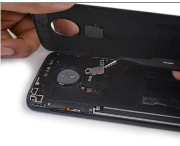
• Use a pair of tweezers to remove the fingerprint sensor cable retention bracket.
