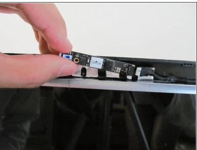
Carefully disconnect the camera board from the laptop. We used tweezers.
