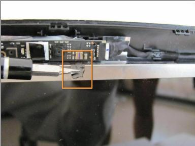
Remove the 2 pieces of black tape using a sharp tool to free the camera board, note that the camera board is still connected to a cable.
