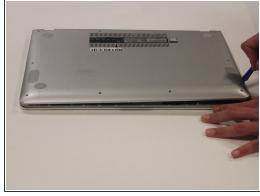
Use the plastic opening tool to gently pry the back cover of the laptop up. Slide the tool slowly along the edges of the back cover to pop it out of the clips holding the cover in place.
