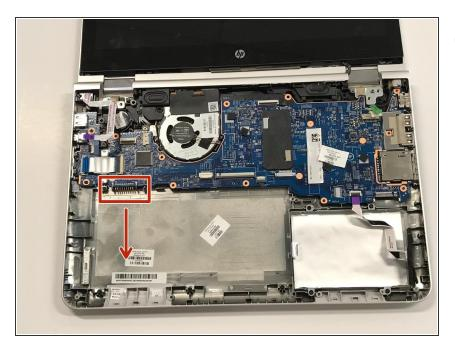
Gently lift the battery and bring downward away from its port to remove it from the laptop.
