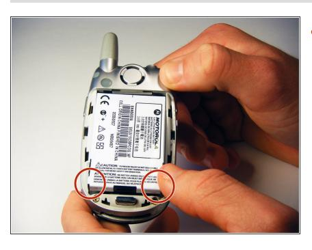
Lever the battery out by pressing upwards on the bottom corners of the battery.
