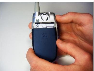
Press down on the chrome button on the bottom of the chassis. Simultaneously slide the back cover down, away from the phone.
