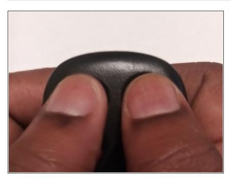
Press the lock and unlock buttons on the key fob simultaneously until the vehicle automatically locks and unlocks (This can take approx. 30 secs.)
