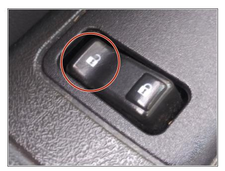
Release the unlock button on the driver side door. You should hear the vehicle automatically lock and then unlock.
