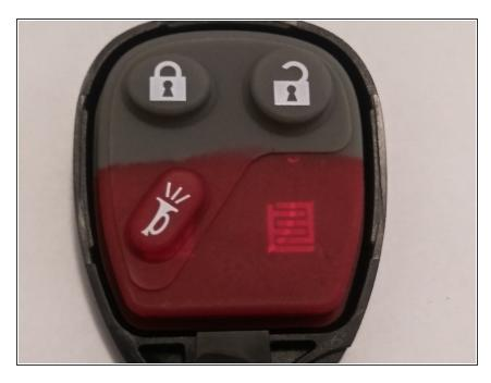
To remove the buttons, lift the "rubber button pad" from the key fob shell.
