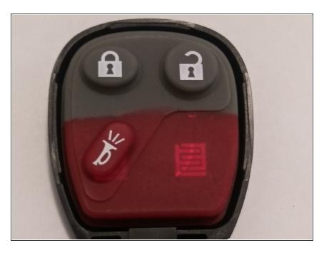
Insert rubber button pad over the battery. Place the front end of the key fob over the buttons and press down until you hear a "click".
