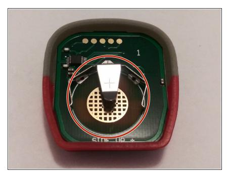
Remove the old CR2032 battery by simply pulling it out and replace it with a new one.
