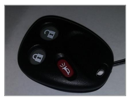
Use the spudger to pry open the key fob shell by sliding it in between the front and back part of the key fob.
